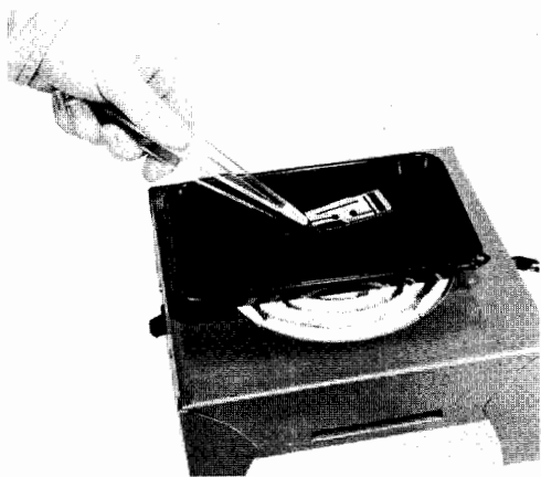
Fig. 60—Hot etching of printed-circuit board.
