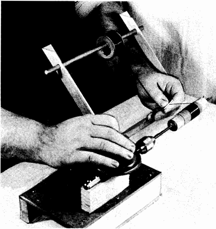
Fig. 100—Over-all view of the home-built coil-winding jig in operation. A "guide-paddle" is used to ensure level winding and professional appearance.
