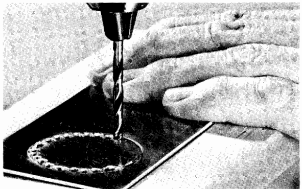
Fig. 45—Four ways to drill large holes.
