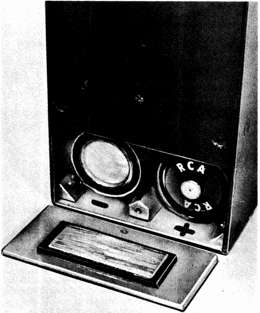
Fig. 166—Battery compartment with batteries installed.
