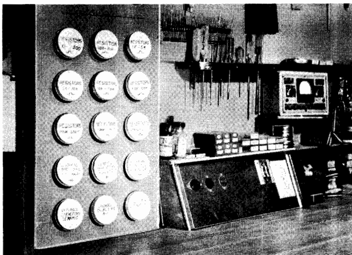
Fig. 80—Rack for storage jars can be made from plywood panel, Masonite, or scrap wood.
