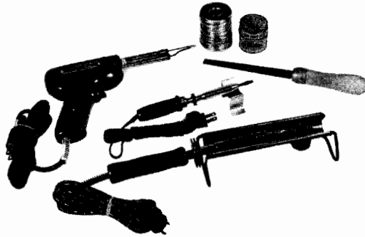
Fig. 3—General-purpose soldering gun at top has built-in spotlight. Small soldering iron at center is useful for printed circuit work and miniaturized projects. Large iron at bottom is suitable for most types of electronic work.
