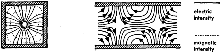
Fig. 6 —Instantaneous field configuration for a TM_{1,1} wave.
