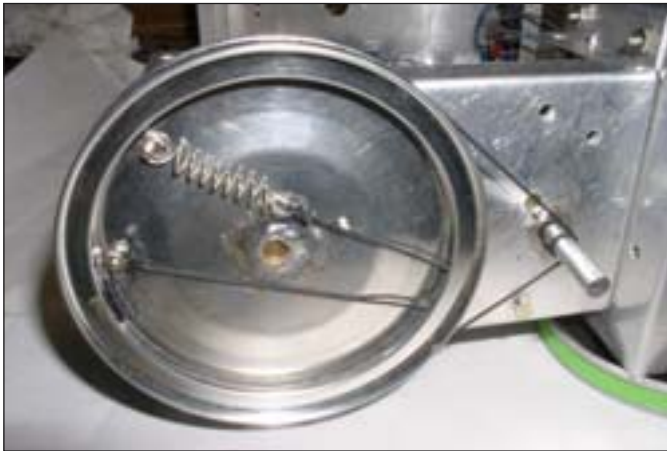
Fig 13 —The dial-cord routing: 1½ turns around the drive shaft, 2 turns around the drum with the ends through the slot. One end of the cord attaches to one of the machine screws opposite the drum cylinder slot. The other end ties to a spring attached to the other screw.
