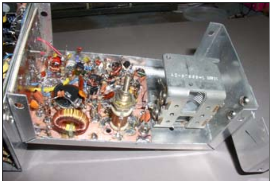
Fig 8—The VFO tuning capacitor inside, mounted on the front of the more-rigid box section that has the folded tabs.
