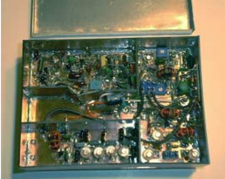
The completed SSB generator. An aluminum lid fits over the top of the box.
