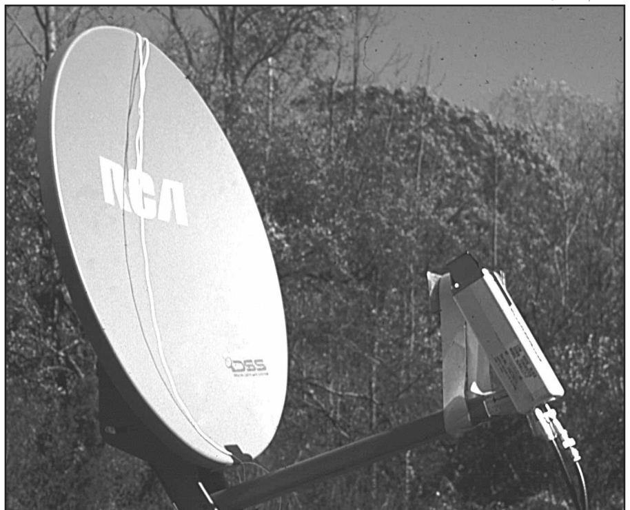
Figure 2—An 18-inch DSS offset dish antenna modified for use on 10.5 GHz.
