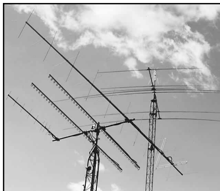
Figure 1—When you think of satellite antennas, this is the image that usually comes to mind. Notice that the antennas on either side of the horizontal boom are crossed Yagis—they have horizontal and vertical elements. (The big HF beam in the background is still waiting for the sunspots to return!)
