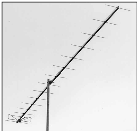
Figure 2—A long-boom horizontally polarized 70-cm Yagi will also work for Phase 3D; its extra gain is largely negated by the polarization mismatch, and the higher gain makes it more difficult to point.
