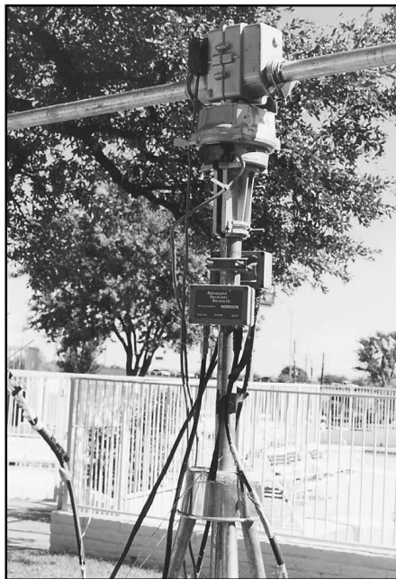
Figure 3—This ground-mounted antenna installation uses an azimuth/elevation rotator system. The horizontal antenna boom is connected through the elevation rotator (top). Notice the receive preamplifier (an Advanced Receiver Research model) below the rotators.
