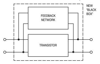
For example, the above combination of transistor and feedback network may be characterized as a single "black box" by the following equations:<sup>†</sup>
