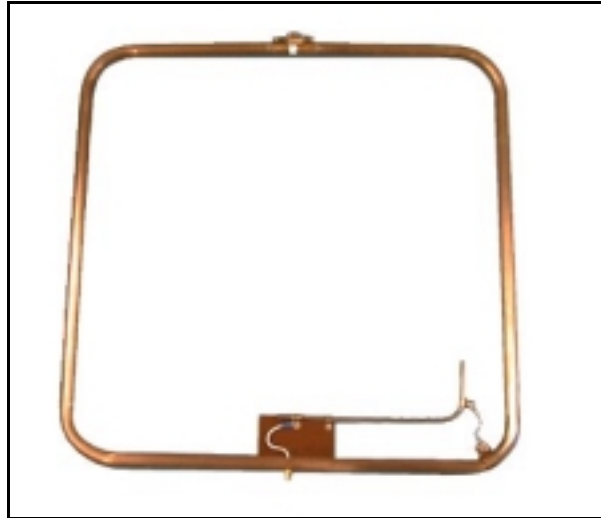
Figure 4. Copper Tube Antenna 500mm x 500mm
