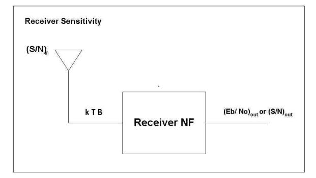
$$\begin{split} (S/N)_{in} &= (S/N)_{out} + NF\\ S_{in} - N_{in} &= (S/N)_{out} + NF\\ S_{in} &= N_{in} + (S/N)_{out} + NF\\ \end{split}$$
