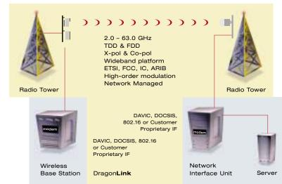
DragonLink employs the latest MMIC and packaging technology coupled with a low-cost topology to provide a fully optimized solution. The system includes both base station and Customer Premise Equipment (CPE) radios which can be purchased as a set or engineered to interoperate with other radio equipment such as third-party base station radios.
