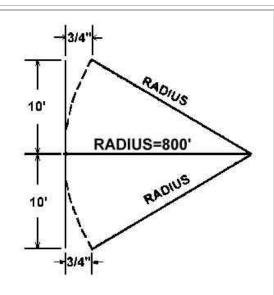
Radius of curvature is meant to be a definition of points on the surface of a circle. A radius of 800' represents a <sup>3</sup>/<sub>4</sub>" deflection from a tangent line to a circle over 10' increment. Radius of curvatures should be above 800' at maximum design wind loads.
