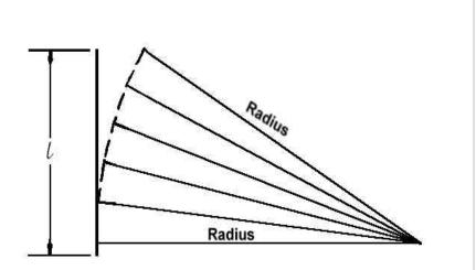
To determine minimum radius of curvatures, several points along the antenna length should be taken. Points at 5' increments are satisfactory.
