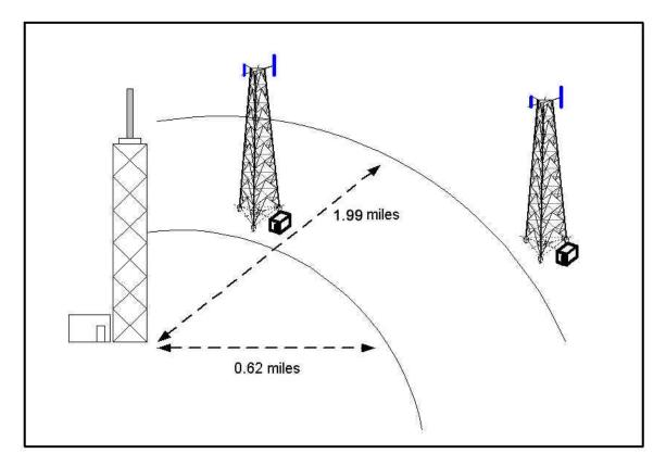
Base station towers close to AM towers can act as a reflector for the AM transmitting antenna and change its existing coverage.
