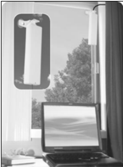
Photo 2-5: Antenna on Residential Window
