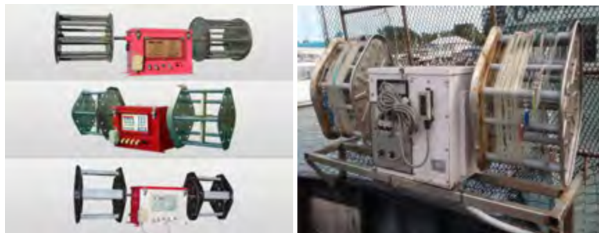
Gambar 166. Mesin pancing cumi otomatis (jigging automatic machine)
